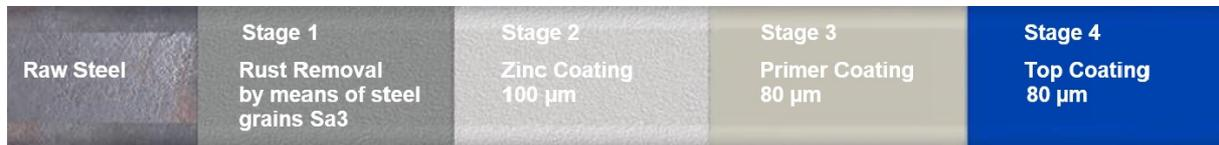
The coating thickness is 260 µm, all requirements on corrosion protection stresses according to DIN EN 12944-2- C4 (long protective effect) are met.
