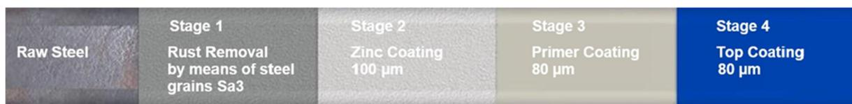
The coating thickness is 260  $\mu$ m, all requirements on corrosion protection stresses according to DIN EN 12944-2 of the category C4 (long protective effect) are met.
