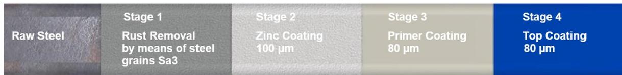
The coating thickness is 260 µm, all requirements on corrosion protection stresses according to DIN EN 12944-2 C4 (long protective effect) are met.
