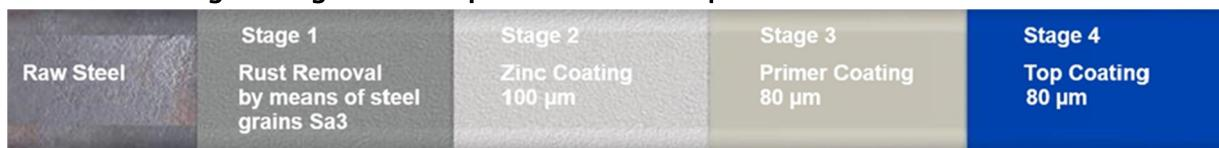
The coating thickness is 260 µm, all requirements on corrosion protection stresses according to DIN EN 12944-2 of the category C4 (long protective effect) are met.
