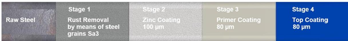
The coating thickness is 260 µm, all requirements on corrosion protection stresses according to DIN EN 12944-2 of the category C4 (long protective effect) are met.
